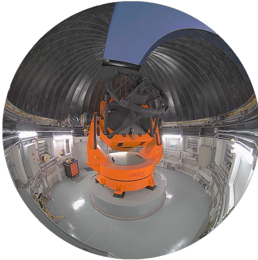
The COLIBRI ground-based telescope in its dome. Its performance, combining excellent sensitivity, remarkable speed and coverage of wavelengths from the visible to the near infrared, is unique at international level. The telescope and its dome can observe on any part of the sky in fewer than 20 seconds, making COLIBRI the fastest telescope in its category. © COLIBRI&A. Watson, UNAM
