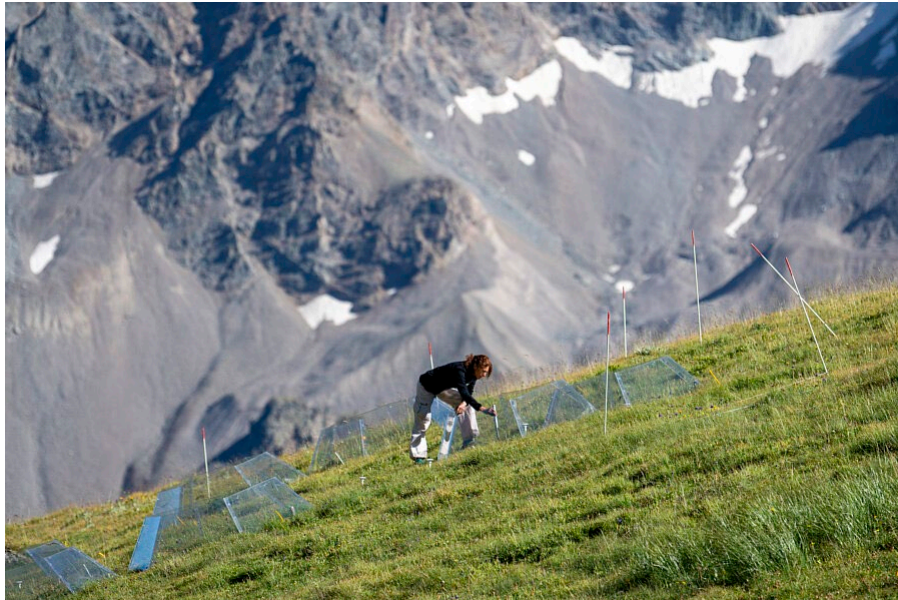
Sandra Lavorel, the winner of the 2023 CNRS Gold Medal, surrounded by the equipment used in the Warm project, which studies the effect of climate change on alpine grass. Installed at the Col du Lautaret at an altitude of 2,400 m, they heat the air a few degrees in relation to the external temperature in order to study the consequences on the ecosystem (production of biomass, temperature, and soil humidity).
