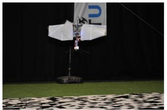
Flapping-wing robot controlling its attitude using this new principle. It is equipped with an artificial compound eye inspired by insects, which can perceive optical flow at a high frequency. © Christophe De Wagter/TU Delft
