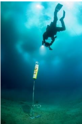
A diver checks and retrieves a hydrophone under the sea ice off Adélie Land. © Erwan Amice / LEMAR / CNRS Photo Library
