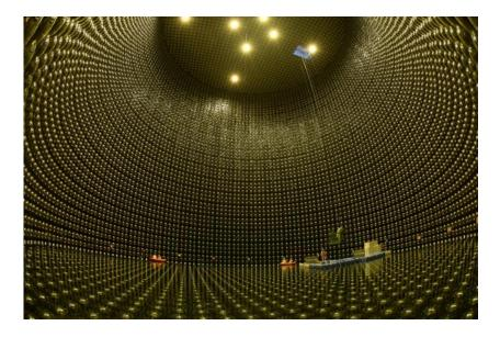
The Super-Kamiokande detector is a tank 40 metres high and 40 metres in diameter, filled with 50,000 tonnes of ultra-pure water, and carpeted with 13,000 detectors.
