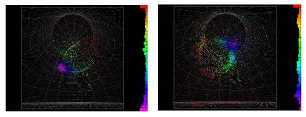
Detection of an electron neutrino (on the left) and an electron antineutrino (on the right) in the Super-Kamiokande. When an electron neutrino or antineutrino interacts with water, an electron or a positron is produced. They emit a faint ring of light (called Cherenkov light) that is detected by almost 13,000 photodetectors. The colour on the figures shows how photons are detected over time.
