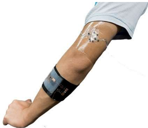
Image of the wearable biofuel cell applied to the arm, powering a diode attached to the black armband on the forearm. © Xiaohong Chen, Département de chimie moléculaire (CNRS/Université Grenoble Alpes)
