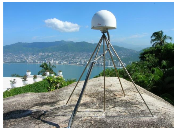
Two permanent GPS stations , one on the roof of the school in Papanoa, the epicenter of the April 2014 earthquake (PAPA station, left), while the other is at the center of the Guerrero seismic gap, overlooking Acapulco bay (ACAP, right).
