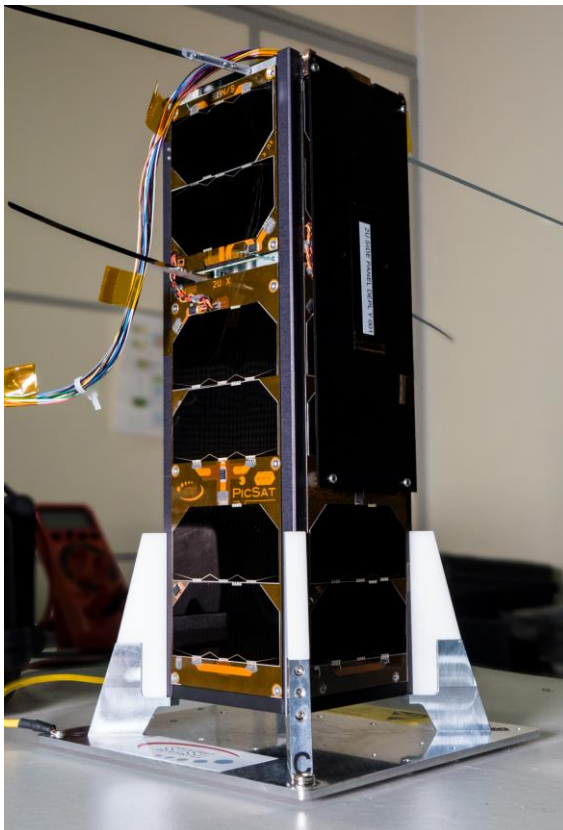
PicSat, with its unfolded antennas, in the lab's vacuum chamber © LESIA / Observatoire de Paris-PSL
