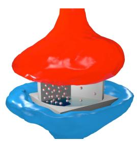
Artist's impression of the electronic synapse: the particles represent electrons circulating through oxide, by analogy with neurotransmitters in biological synapses. The flow of electrons depends on the oxide's ferroelectric domain structure, which is controlled by electric voltage pulses. © Sören Boyn / CNRS/Thales physics joint research unit.
