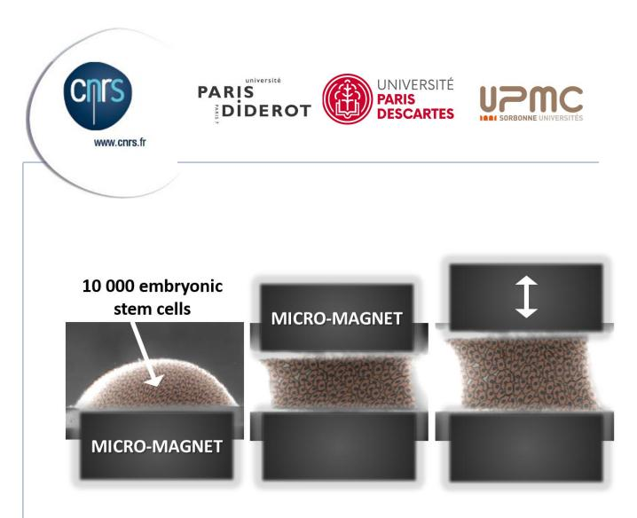
The magnetic stretcher: this all-in-one system can both form and mechanically stimulate an aggregate of embryonic stem cells. The two micromagnets, one of which is mobile, frame the resulting embryonic body, and cyclical stimulation can be adapted to the type of tissue being sought. © Claire Wilhelm / Laboratoire Matière et systèmes complexes (CNRS/Université Paris Diderot).
