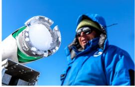
Sampling of an ice core during the testing of the prototype of the Mini-Subglacior experimental probe on the Concordia station in Antarctica. Within a single field season (2 to 3 months), the Subglacior probe will make it possible to explore the ice up to 3 km deep to obtain climatic recordings of the last 1.5 million years, the oldest data obtained from natural ice. © Thibaut VERGOZ / IPEV / LGGE / CNRS Photo library
