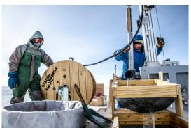
First test of the prototype of the Mini-Subglacior experimental probe on the Concordia base in Antarctica. The engineers are checking that the ice chips rise to the surface correctly.
