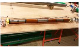
The OF-CEAS laser spectrometer embedded inside the probe. The instrument itself is only 40 mm in diameter. It is inserted here in a vacuum pressure tube with a diameter of 50 mm
